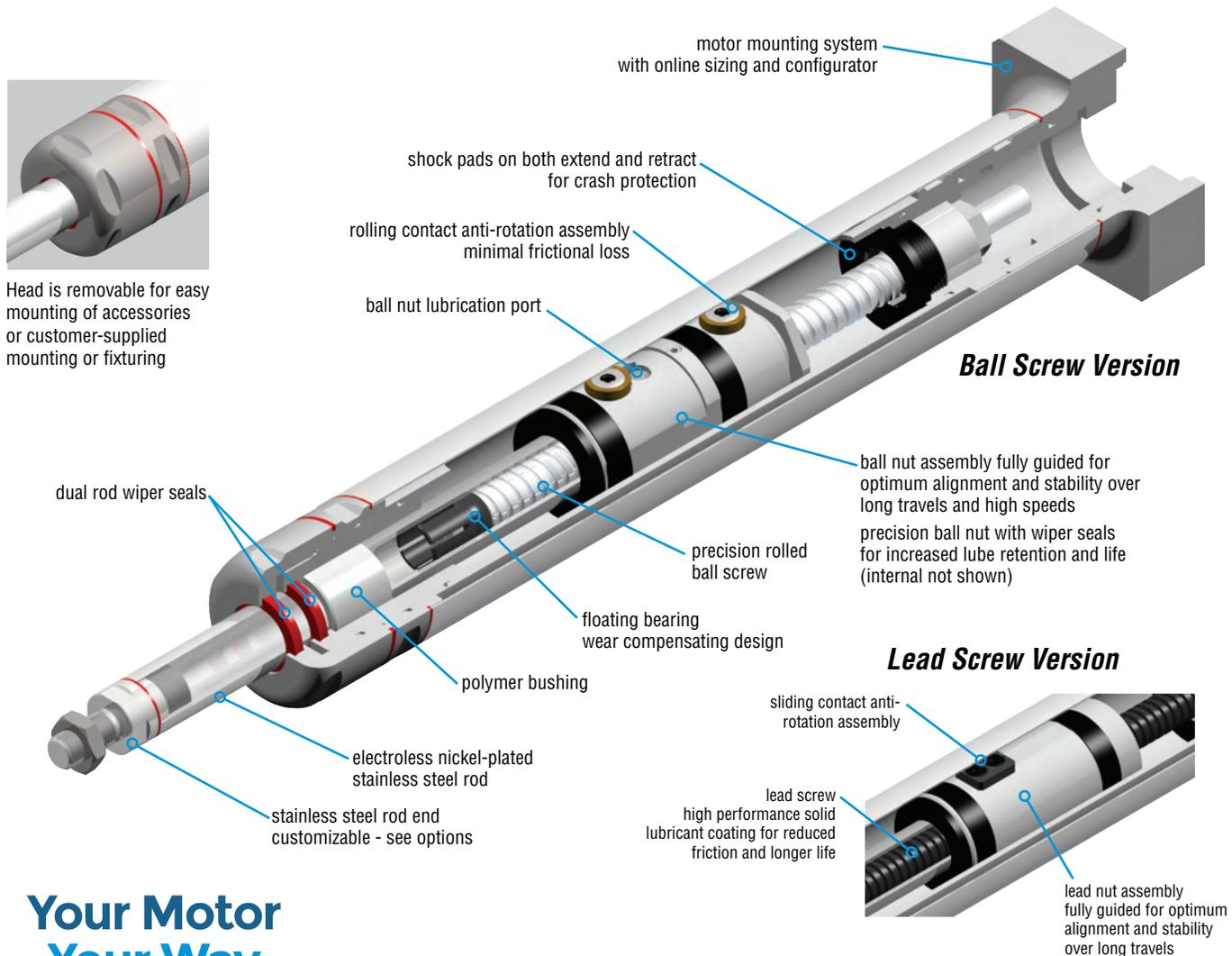
Head is removable for easy mounting of accessories or customer-supplied mounting or fixturing
