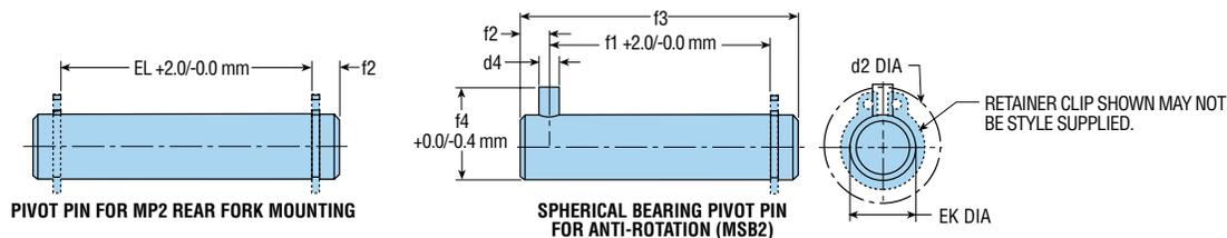
PIVOT PIN FOR MP2 REAR FORK MOUNTING
