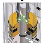
All PHD swing arm clamps are rotated into position by three hardened steel balls running against a hardened steel spline. This superior design outlasts the competitor's single pin design.
